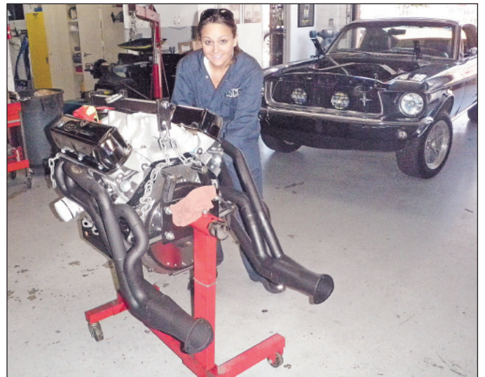
FITTING THE NEW HEADERS ON THE 392 CI CRATE FORD 430-HORSE RACING ENGINE
